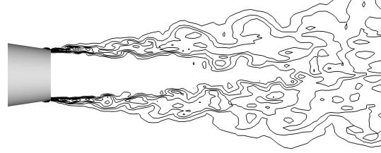
(b) Jet III (Synthesized inlet turbulence)
